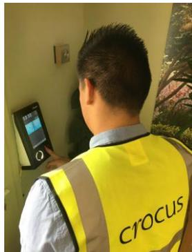
Bodet installed 5 of their latest Kelio Visio X7 smart terminals, each featuring both a biometric and proximity reader. These all interface with cloud-based Time & Attendance software.
